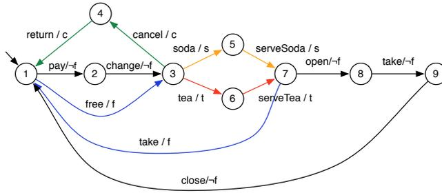
Fig. 2: VIS Feature Transition System of a beverage vending machine [24, 30]
