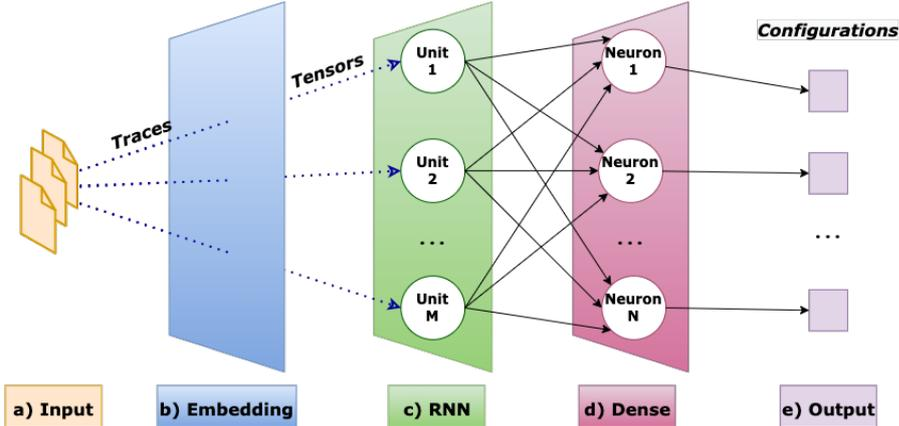
Fig. 4: Description of the VaryMinions architecture
